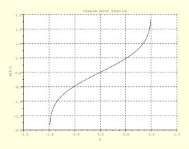
erf<sup>-1</sup> is the inverse of the normalized error function erf(x)  $\equiv \frac{2}{\sqrt{\pi}} \int_0^x e^{-u^2} du$
